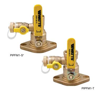
\*This valve is designed to be soft soldered into lines without disassembly, using a low temperature solder to 420°F (216°C). Higher temperature solders may damage the seat material.
