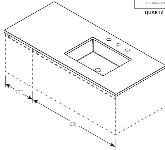
**Note:** Sinks must be located over H1-Tip Out or H2/V14 Plumbing drawers. See Cartesian Reference Guide for more information.
