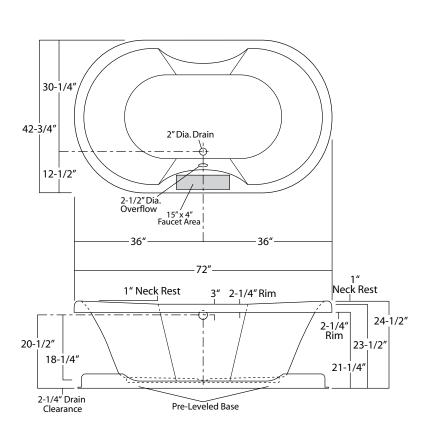
Sump Dimen: 50" long x 28" wide x 20-5/8" deep Sump Capacity: 88 gal. (unoccupied - to overflow)
