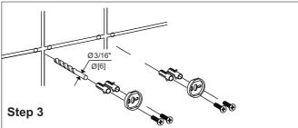
Predrill 3/16" holes on the wall to fit wall plugs. Insert wall plugs into the wall. Position backing plates flat side down over the plugs and install screws.
